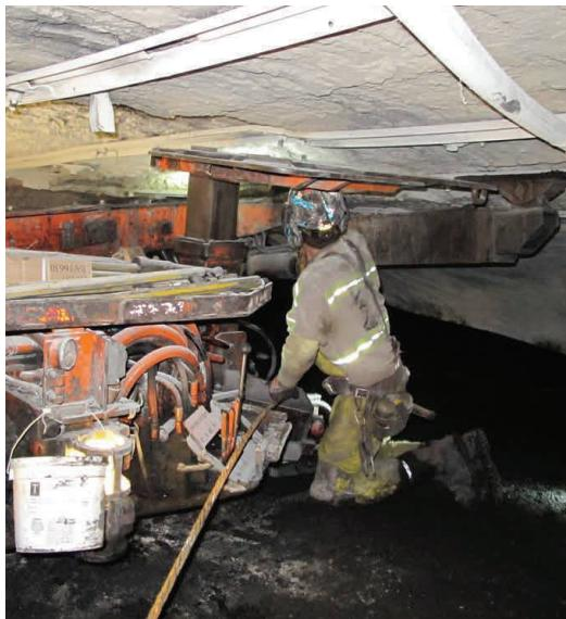
Cable bolt usage is increasing—and so is the chance of the long cable bolt accidentally activating the controls
